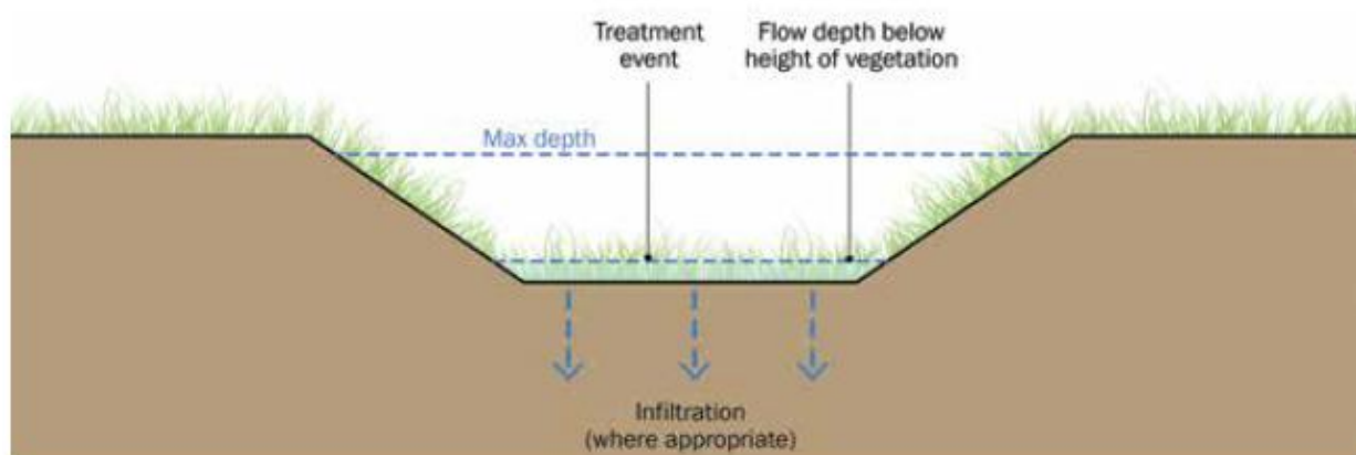
Figure 6-3: Swale: Conceptual Design Details
